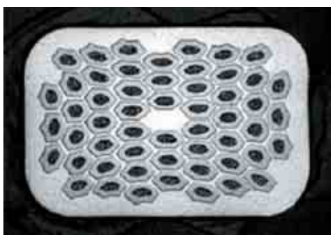
写真5 Ta-Sn 粉末法 Nb 3 Sn 線材の断面 Photo 5 Cross-section of Ta-Sn powder-in-tube processed Nb 3 Sn superconductor
