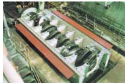
写真 1 鋳鋼製組立型クランク軸 Photo 1 Semi-built-up type crankshaft made of cast steel
