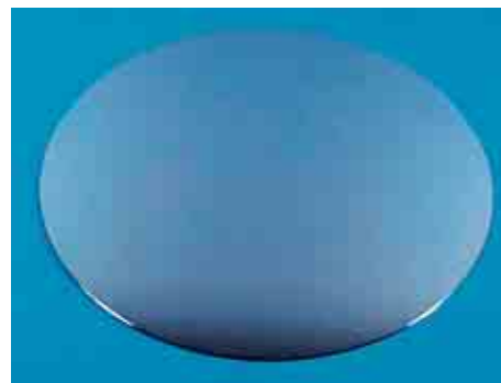
写真2 銅濃度0.2%で人為的に汚染させた開発溶液に10分浸漬したウェーハ Photo 2 Wafer immersed in developed etching solution intentionally contaminated with 0.2% of copper for 10 min
