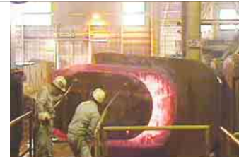
Throw : checking alignment by using steel board
