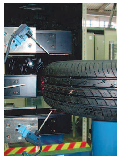
図12 乗用車用タイヤ向け試作センサ Fig.12 Prototype sensor for passenger car tires
