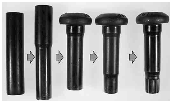
図10 トルシア形高力ボルトの各工程の外形 Fig.10 Shapes after each stage of torshear type high-strength bolt
