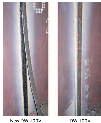
図7 スラグ剥離外観の比較 Fig. 7 Comparison of slag detachment between DW-100V and conventional one
