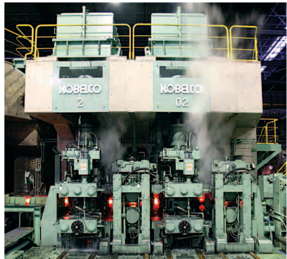
図4 NKCS ミル (New KOBELCO Compact Solid Mill) Fig. 4 NKCS Mill (New KOBELCO Compact Solid Mill)
