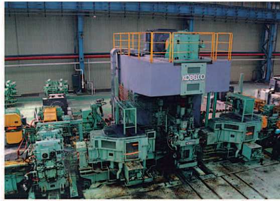
Finishing mill train
