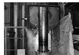
Ingot produced by EB ( 220 x L1,500mm, 450kg)
