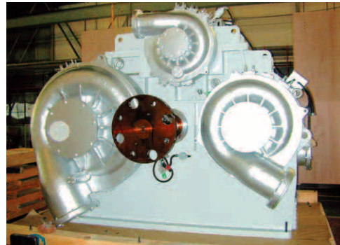
図1 3ピニオン6段階増速機内蔵型遠心圧縮機 Fig. 1 3 Pinions - 6 stages integrally geared centrifugal compressor
