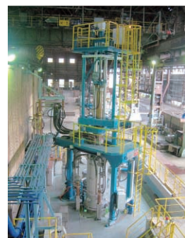
図1 最新鋭ESR炉 Fig. 1 State-of-the-art ESR furnace
