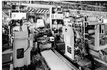
図8 新内部欠陥探傷装置 Fig. 8 New ultrasonic testing system
