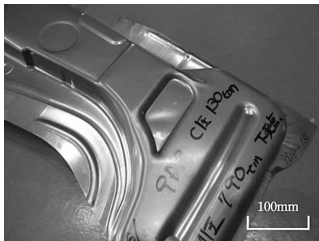
図12 プレス品のしわ (BHF=1,300kN) Fig.12 Example of wrinkle in test part (BHF=1,300kN 980DP steel)
