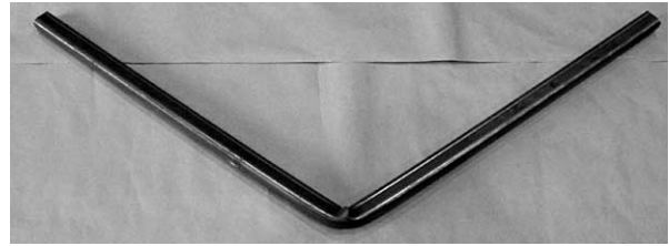
図10 300mm 押し込み後の開発ドアビーム Fig.10 Developed beam after device 300mm stroke
