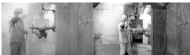
図10 エアスプレー塗装(左)と静電塗装(右) Fig.10 Air spray painting(left) and electrostatic painting(right)
