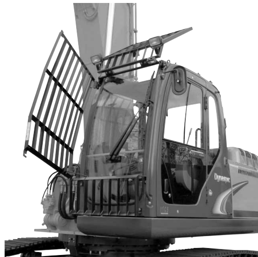
図13 解体キャブ外観 Fig.13 Appearance of demolition cabin
