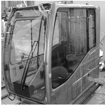
図9 キャブ打撃試験 Fig. 9 Impact hammer testing of cabin
