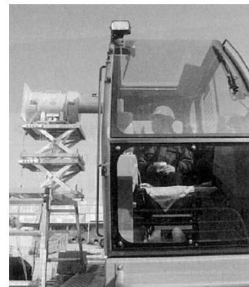
図11 キャブの気密度計測 Fig.11 Measurement of airtightness of cabin
