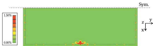
図15 ルーフパネルの相当塑性ひずみ分布 Fig.15 Distribution of equivalent plastic strain in roof panel
