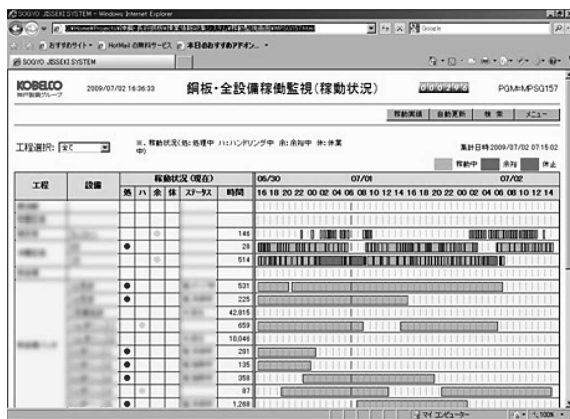
図3 全設備稼働監視画面 Fig. 3 Operation monitoring of all equipments
