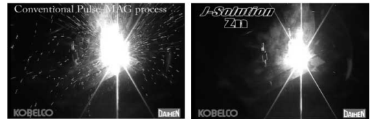
図22 J-Solution Znの低スパッタ効果 Fig.22 Reduction of spatter generation by J-Solution Zn
