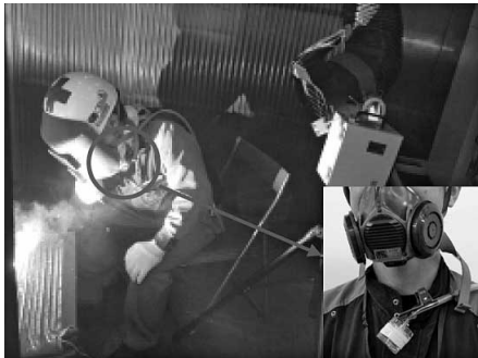
図11 Cr(VI) 暴露量測定風景 Fig.11 Measurement of Cr(VI) exposure
