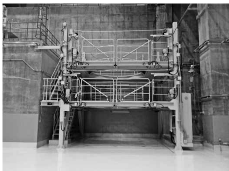
図10 検査架台 Fig.10 Deck frame for testing
