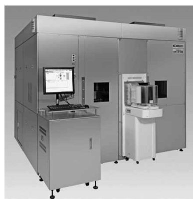
図1 LSW-3010FE (サブナノ精度サイトフラットネス計) 2) Fig.1 LSW-3010FE (Site flatness measurement system with an accuracy of sub-nanometer order for silicon wafer) 2)
