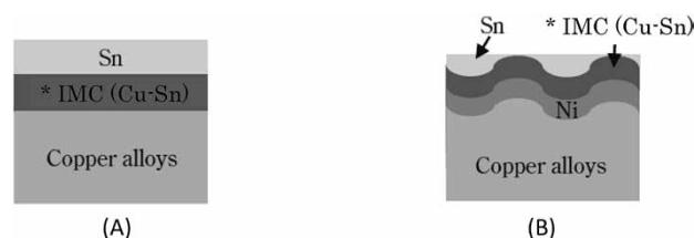
図3 すずめっき付銅合金の断面構造の概略 Fig. 3 Schematic image of cross-section of tin plated copper alloy (A) Reflowed tin plating, (B) New-reflowed 3 layer tin plating with Ni undercoat *IMC: intermetallic compound layer of Cu and Sn
