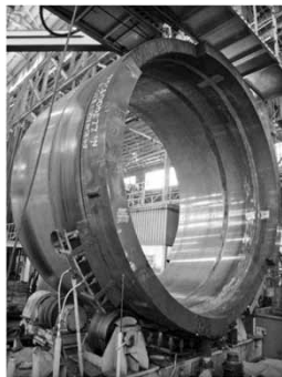
図10 9Cr-1Mo-1/4V-Nb鍛造鋼製シェルリング Fig.10 Forged shell ring made of 9Cr-1Mo-1/4V-Nb steel
