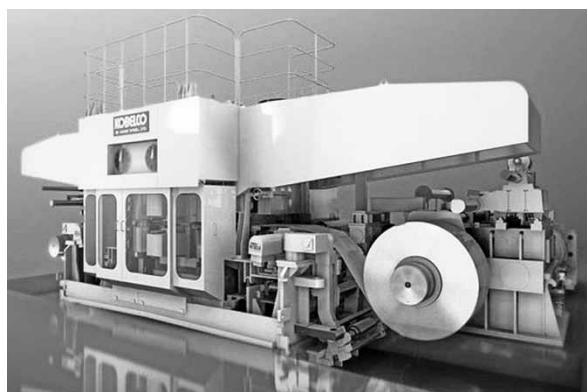
図1 KTミル全体図 Fig. 1 General view of advanced KT mill
