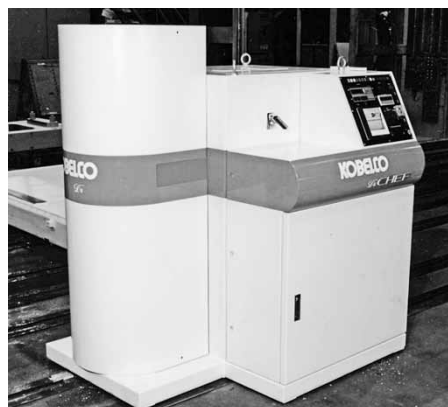
図3 研究開発用食品高圧処理装置 (Dr.CHEF) 1) Fig. 3 High pressure food processing equipment for R&D (Dr.CHEF) 1)
