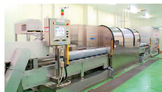
図2 食品高圧処理用横型CIP装置FOOD FRESHER Fig. 2 Horizontal cold isostatic pressing equipment for food, "FOOD FRESHER"
