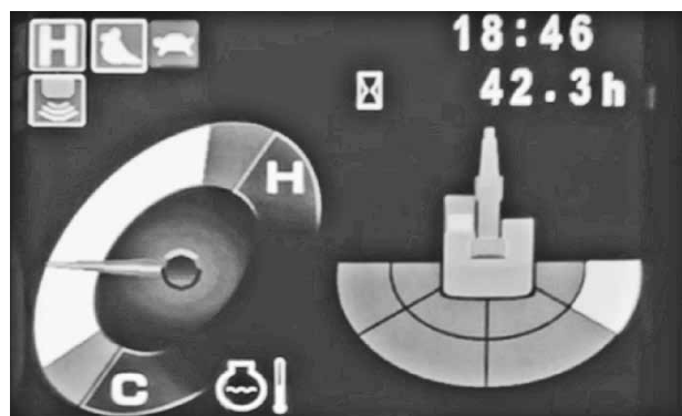
図9 右側方に人・障害物がある場合の表示 Fig. 9 Display in case of being person or obstacle inside deceleration area on the right side of the machine
