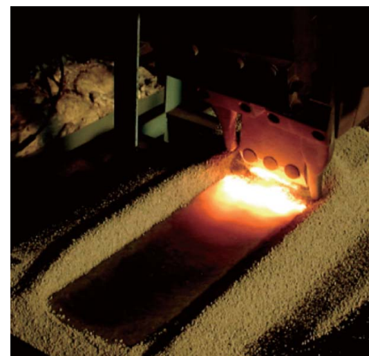
PF-B7FK / US-B309LCb单层堆焊实例 / Overlay welding with PF-B7FK / US-B309LCb
