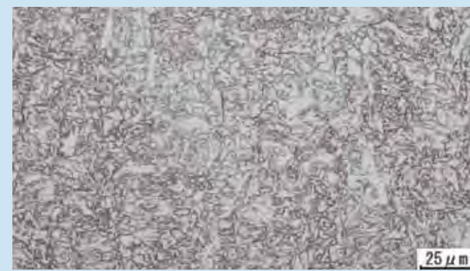
Microstructure of Mn-Mo-Ni steel weld metal
