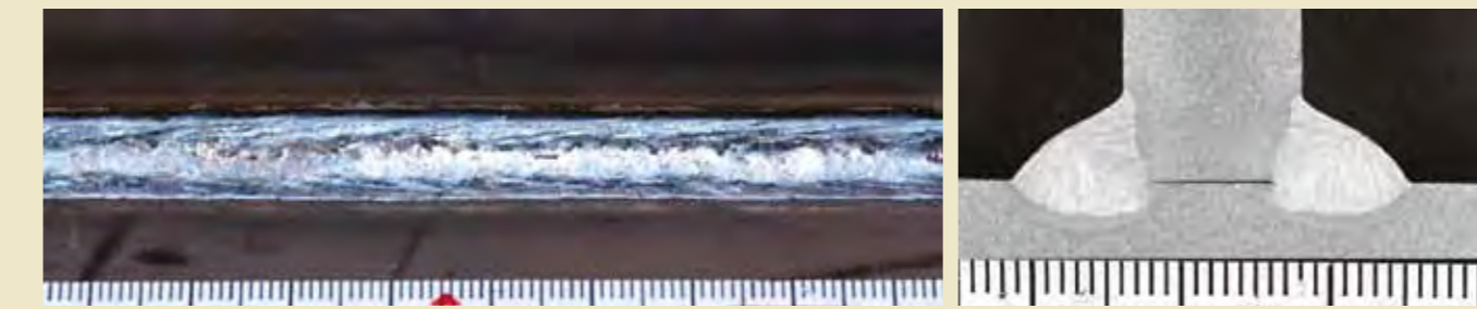
Example of bead appearance and macro structure
