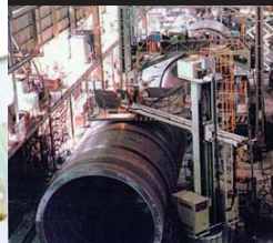
内面の肉盛 (バンド溶接) Strip submerged arc welding for overlay
