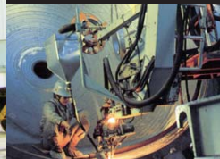
内面の肉盛 (バンド溶接) Strip submerged arc welding for overlay
