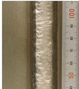
継手のビード外観 Weld Bead Appearance of Butt Joint
