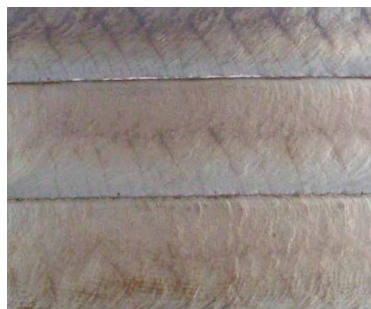
PREMIARC™ PREMIARC™ PF-B7FK / US-B309Lcb 1層肉盛施工例 / Single Layer Overlay with PREMIARC™ PREMIARC™ PF-B7FK / US-B309Lcb
