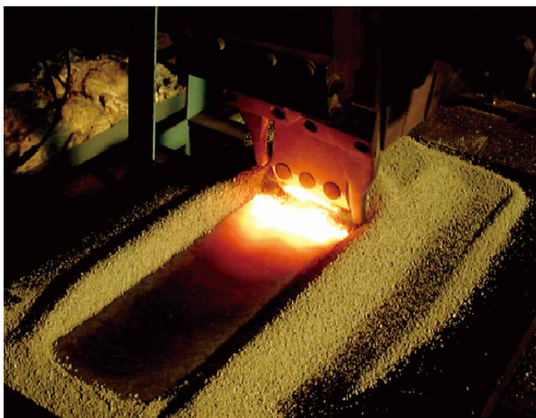
PREMIARC™ PREMIARC™ PF-B7FK / US-B309Lcb 1層肉盛施工例 / Single Layer Overlay with PREMIARC™ PREMIARC™ PF-B7FK / US-B309Lcb
