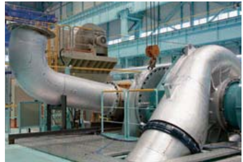
Large-capacity compressor undergoing testing
