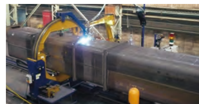
Large-scale column assembly welding system for core columns and connections
