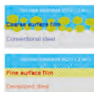
Fig. 1 Schematic illustration of corrosion resistance improvement
