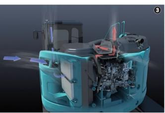
Integrated Noise & Dust Reduction Cooling System (iNDr)
