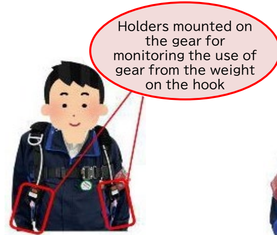
(1) Detection of hook use status
