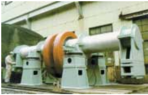
Photo 4 Fatigue testing machine for actual-sized crankthrow
