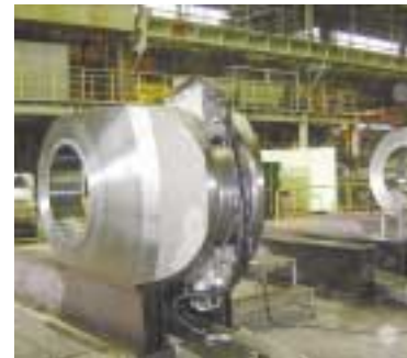
Photo 5 Automatic ultrasonic inspection equipment
