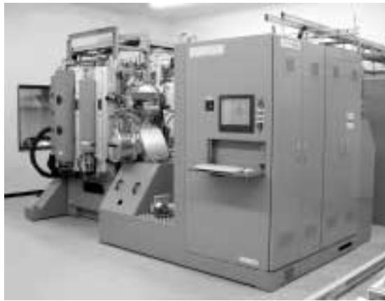
Fig. 2 AIP/UBMS combined system / AIP-S70 Hybrid
