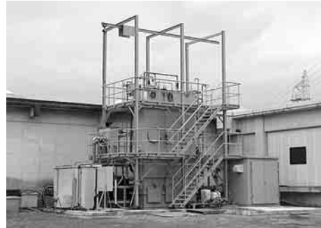
Photo 3 Pilot scale equipment of hollow fiber membrane
