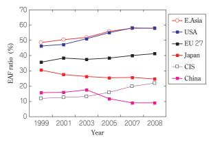
Fig. 7 EAF ratio of crude steel production
