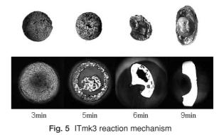
In this new ironmaking process, particles of iron ore and coal exist next to each other in each agglomerate. This is in contrast with the BF and DRI processes, which use bulky materials such as iron ore and coke, and may explain the fast reaction of the new process to some extent. However, this does not fully explain the rapidity of the reactions.
