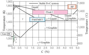
Fig. 1 Operational region of ironmaking processes
