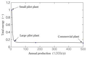
Fig.10 Production size vs. energy consumption
