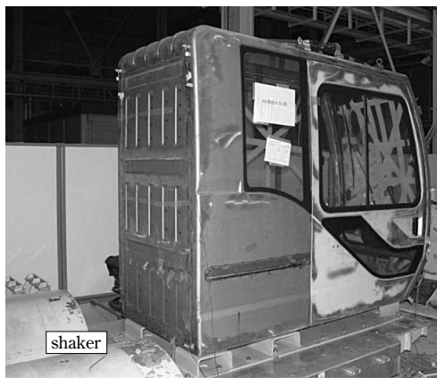
Fig.12 Shaker testing of cabin
