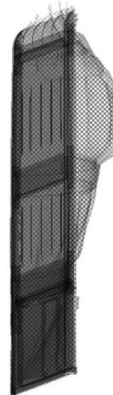
Fig. 7 Mode shapes of rear panel
