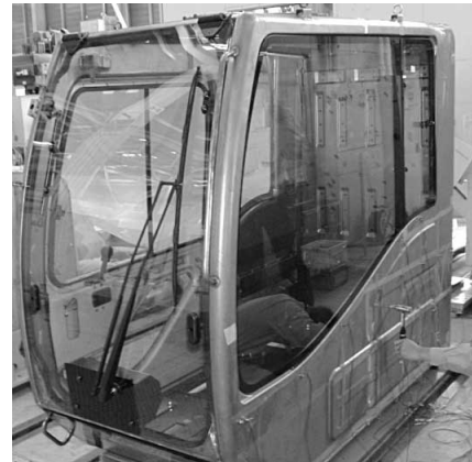
Fig. 9 Impact hammer testing of cabin
