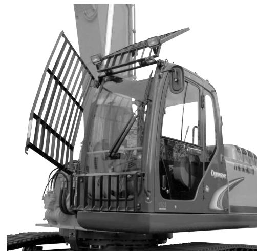
Fig.13 Appearance of demolition cabin
