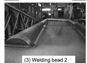
Fig.17 Automatic welding system and welding beads
