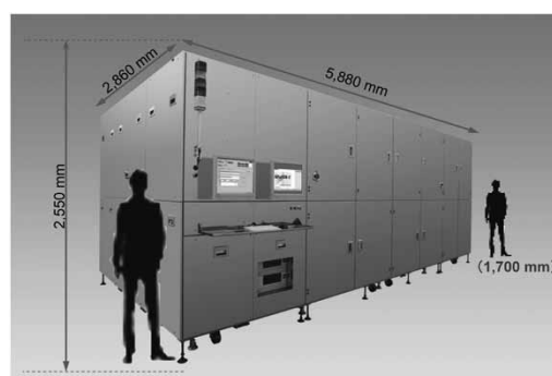
Fig. 1 Evaluation system for oxide semiconductor thin films (LTA-2850SPHIIB: substrate size G8.5)
