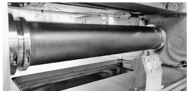
Fig.15 Rotary magnetron sputter source in W35-550CS system
