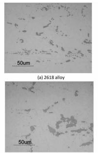
(b) KS2000 under unoptimized condition of homogenization Fig. 4 Optical micrographs of fatigue testing sample
