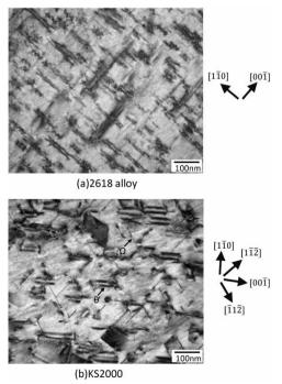
Fig. 2 Transmission electron micrographs after T61 artificial aging followed by exposure at 180°C-400h
