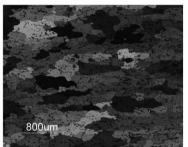
(b) KS2000 under unoptimized condition of forging Fig. 8 Optical micrographs of crystal grain
