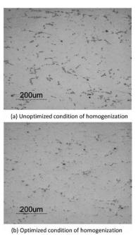
Fig. 6 Optical micrographs of KS2000 forging
