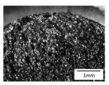
Fig.10 Fractograph in rotary bending fatigue test under optimized condition of forging
