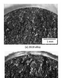
(b) KS2000 under unoptimized condition of forging Fig. 7 Fractograph in rotary bending fatigue tests
