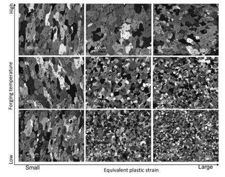
Fig. 9 Influence of crystal grain-size after T61 artificial aging in forging conditions
